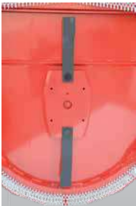
Heavy duty free swinging blades mounted on a high carbon steel rotor protected by an oval stump jumper
