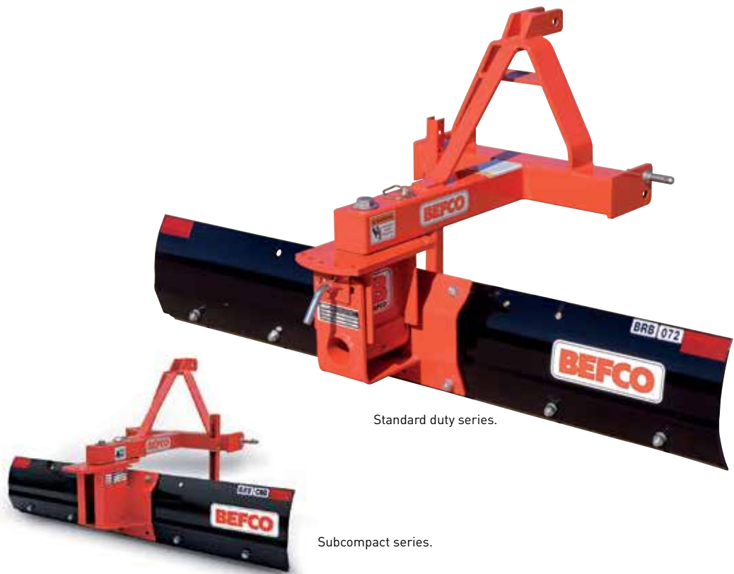
Up to 32° angling on standard duty blades
