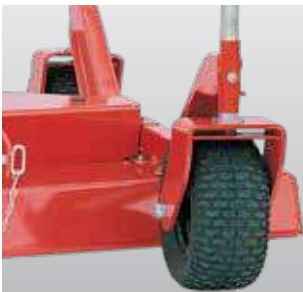
Stamped wheel yoke with choice of hard or air tire
