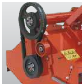
Double belt transmission with automatic belt tensioner
