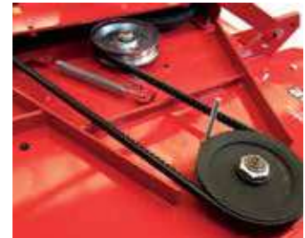
Heavy duty reinforced belt (BX) with automatic belt tensioner
