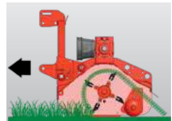
Roller mounted inside the cutting chamber
