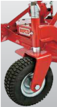
Spacers provide for quick and easy height adjustment
