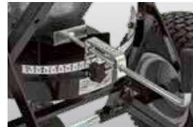
Gate opening control
