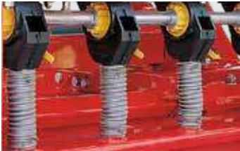
Seed cups for precise metering of seed and fertilizer
