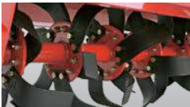
Rotor with 6 blades per flange
