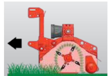
Roller mounted outside the cutting chamber
