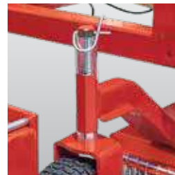
Hexagonal yoke shaft keeps the machine from sliding on hills
