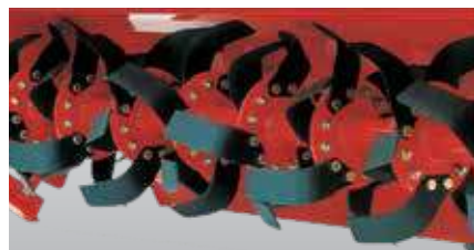
Rotor with 6 blades per flange
