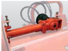
Manual belt tensioning for longer belt life
