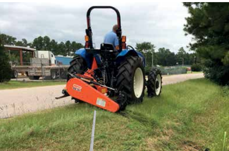
90° up and 55° down mowing capability
