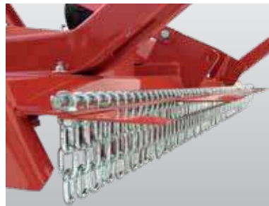
Chains provide safety from thrown objects
